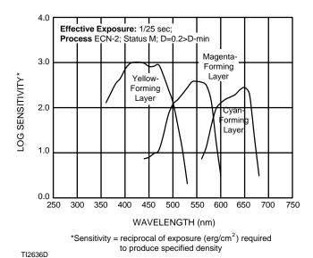
These curves depict the sensitivity of this film to the spectrum of light. They are useful for determining, modifying, and optimizing exposure for blue- and green-screen special-effects work.
